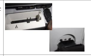
Place an activated transponder in the cradle and check transponder LED is flashing RED, indicating it is charging (the cradle LED should flash alternately GREEN and RED).
